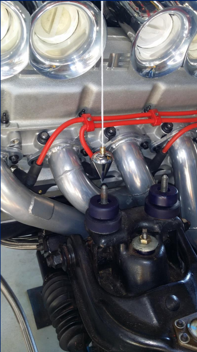
Lining up the K-Frame with the front most mounts..
