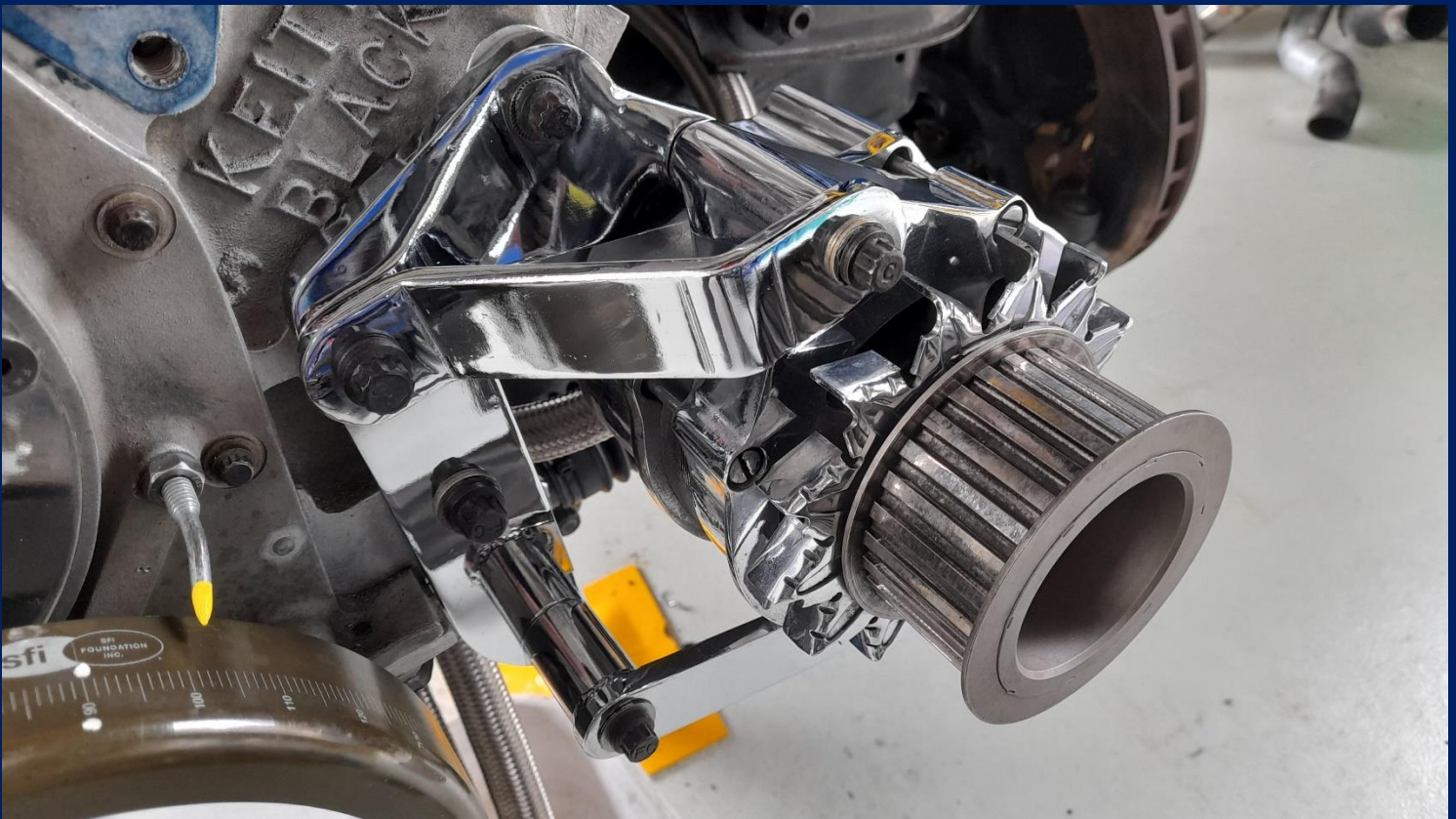
I added some bling with a bit of chrome on the custom alternator brackets..
