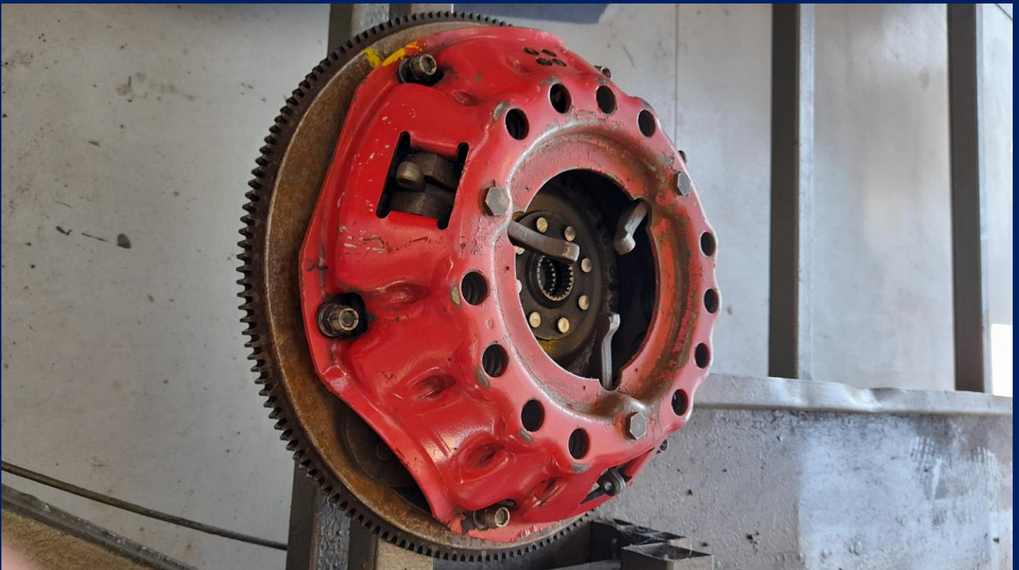
Clutch assembly and flywheel ready for some expert inspection. Luckily all was in great shape, another 20+ years left in the clutch plates (based on current wear rate)!
