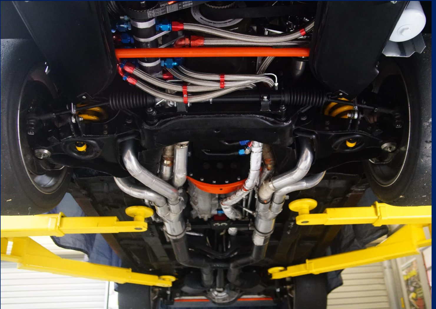
The AXIS TR power steering rack is hidden back there behind the oil and fuel lines
